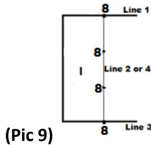
**Step #4** Move line 2 or 4 to tag # **RL** on lines 1 and 3 (**Pic 10**) place spike next to tag **RL** (**Pic 11**). Make sure lines are strait and tight. Now start painting the restraining line by placing your striping machine wheels on the right edge of the line, this keep paint from getting on the lines and tag # (**Pic 12**).
