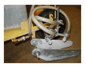
18. By using the right hand control cable you are able to activate the two spray nozzles just like the spray shoe assembly operation.
