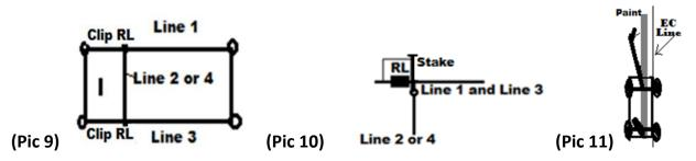
**Step #3** move End line 2 or 4 to clip **RL** on both sides of line 1 and line 3 (**Pic 9**). Place the stakes in the loops right next to the clips **RL** on lines 1 and 3 to mark the top of restraining line (**Pic 10**). Mark a line all the way cross the field. Make sure lines are straight and tight. Now start painting the field by placing your striping machine wheels on the right edge of the line, this keeps paint from getting on the lines and the # Tag (**Pic 11**).
