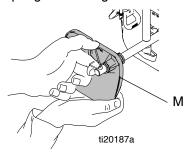
Adjust shields to the desired line width. Spray tip should be centered between shields. Spray pattern should touch shields just above the bottom of the shields.
