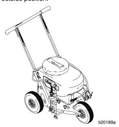
3. Adjust height of tip to adjust line width (raising tip height will create wider lines).
