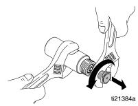
5. Hold CleanShot over running water and clean. Work needle in and out to free CleanShot from excess or hardened material.
