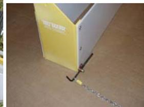
4. The Paint Boom is attached by sliding the square vertical tubular section over the vertical mounting post. The fit should be snug with the painted post.
