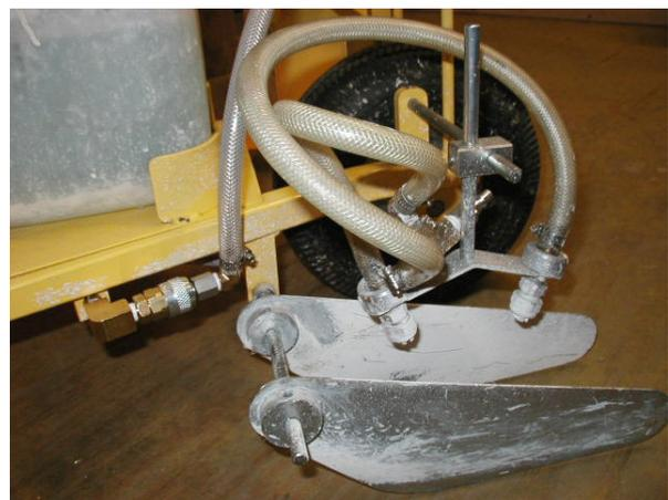
18. By using the right hand control cable you are able to activate the two spray nozzles just like the spray shoe assembly operation.
